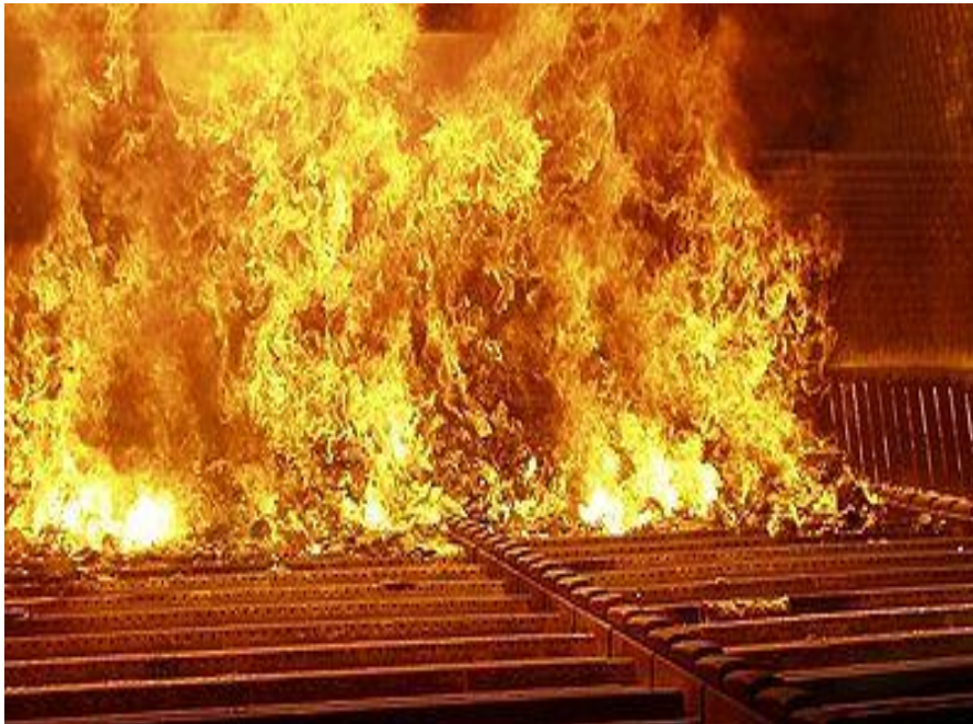
Figure 2.2: Municipal solid wastes in the furnace of a moving grate incinerator capable of handling 15 metric tons (17 short tons) of waste per hour. The holes in the grate elements supplying the primary combustion air are visible. Source: Themelis, Nickolas, (2003)
